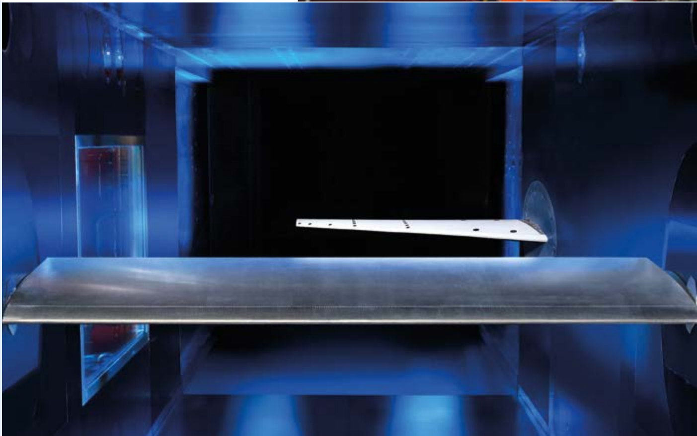
Two-dimensional hydraulically driven profile mounted on the 2D portal support (front) used as a gust generator for a side-mounted three-dimensional wing (background)
