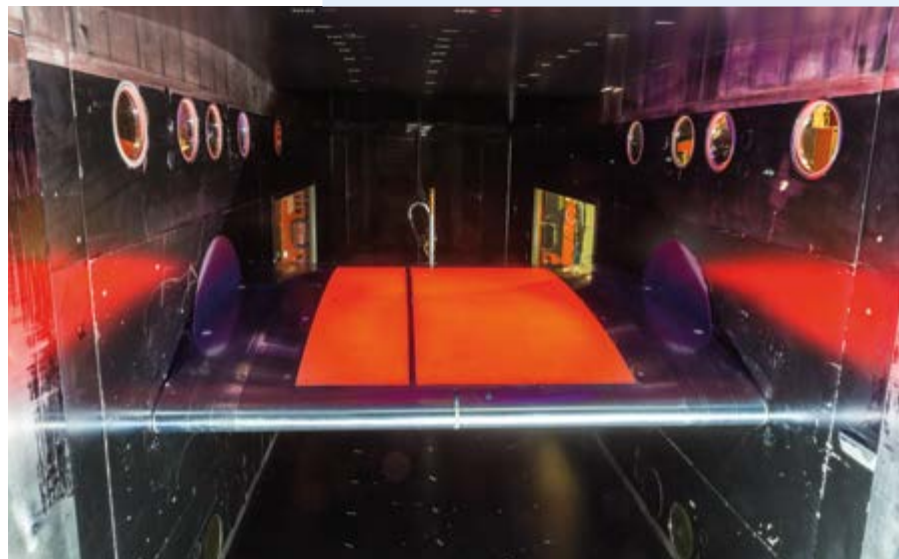
Typical example of method development. Global identification of flow separation and re-attachment for compressible, high Reynolds number flows using Temperature-Sensitive Paint (TSP) during DLR-Project VicToria
