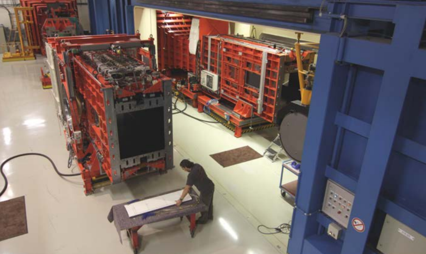
View in open plenum with perforated test-section installed and adaptive and Laval test-section in wind-tunnel hall for preparation purposes
