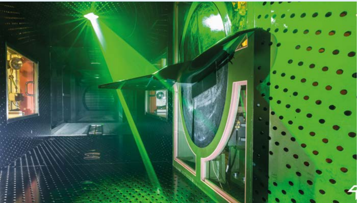
DLR-F23-model in DLR project. PIV is conducted investigating the vortex formation on the upper side of the wing.
