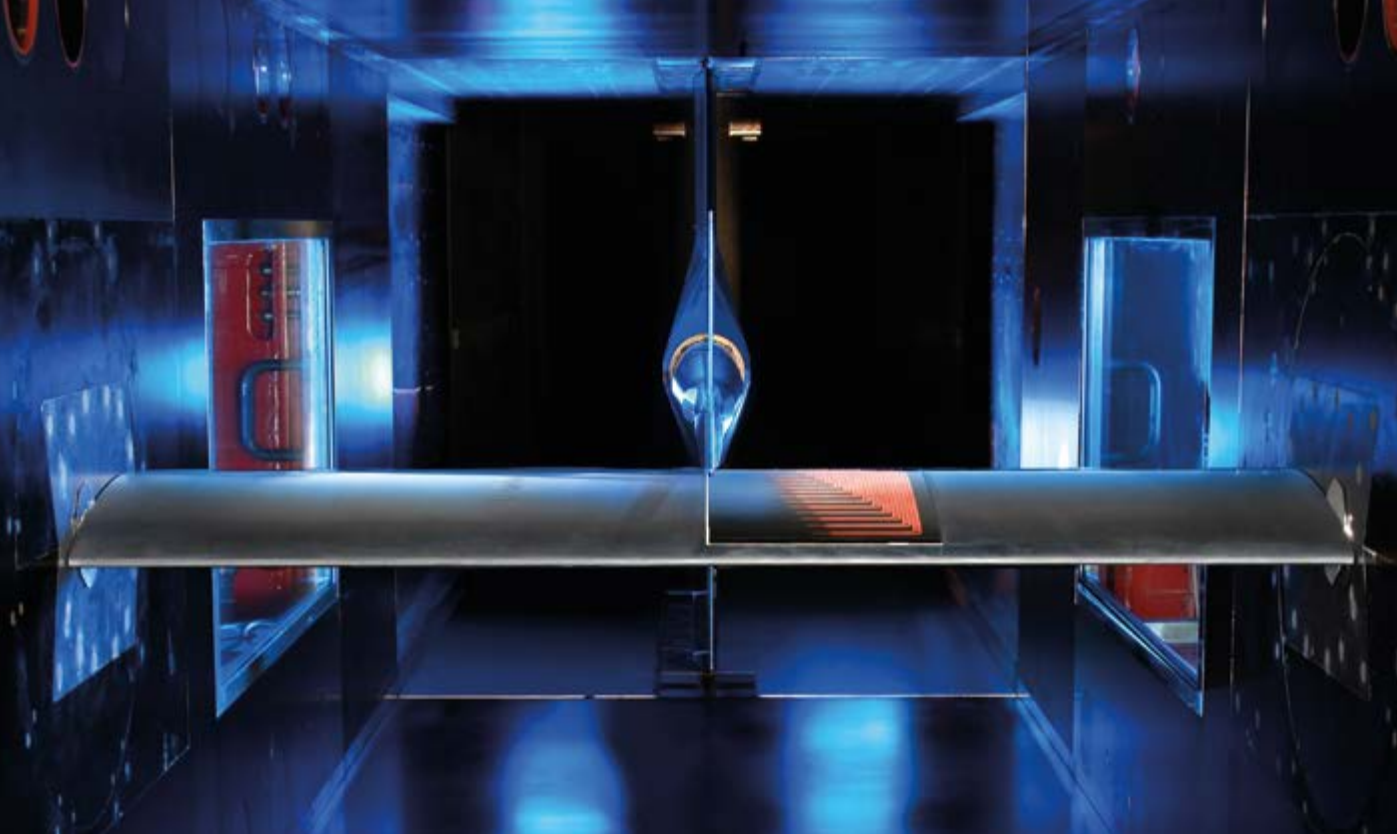
Two-dimensional profile with hotfilm array (front) and wake rake for drag prediction (background) mounted on the 2D portal support of the DNW-TWG
