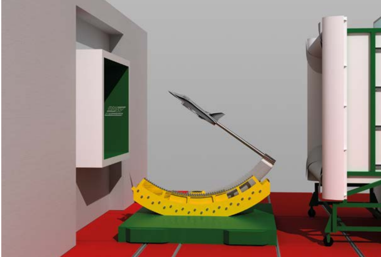
Open test section including rear mounted full model setup
