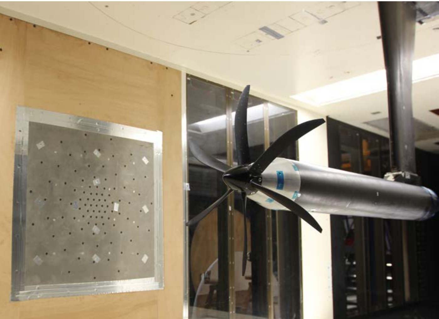
Propeller performance and aero-acoustics; Dowty's baseline propeller design undergoing checkout tests in LST prior to technology development testing in HST & LLF
