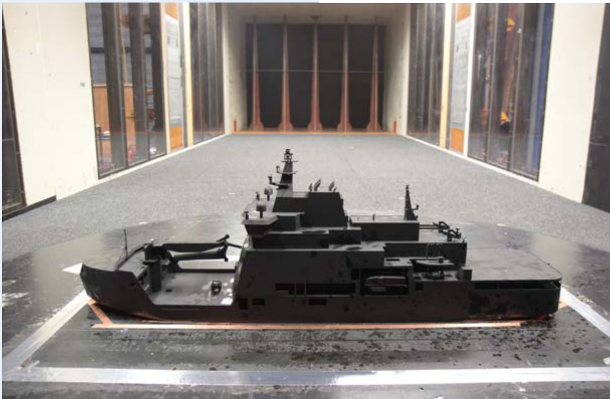
Wind load measurements on a ship
