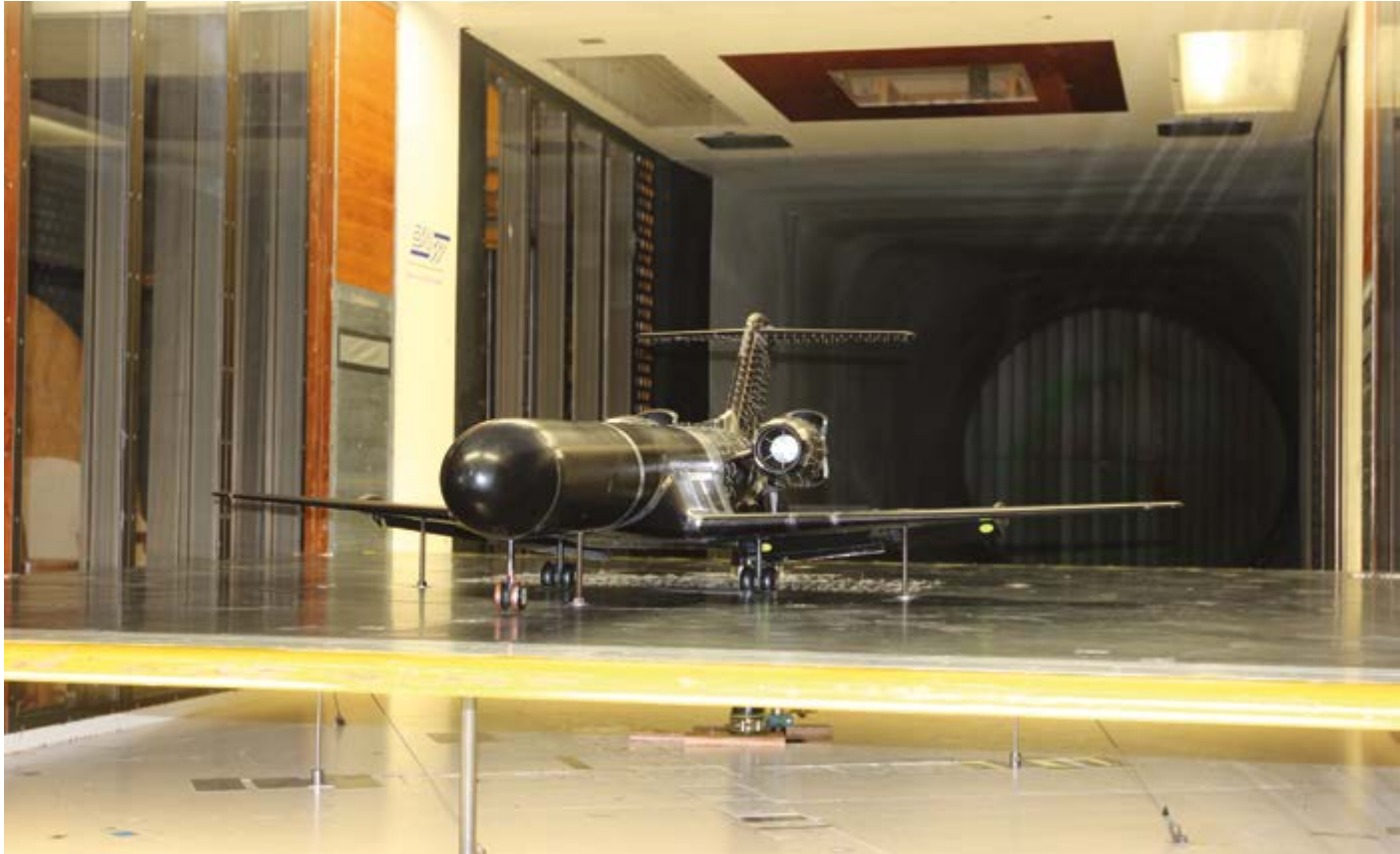
Thrust reverser testing
