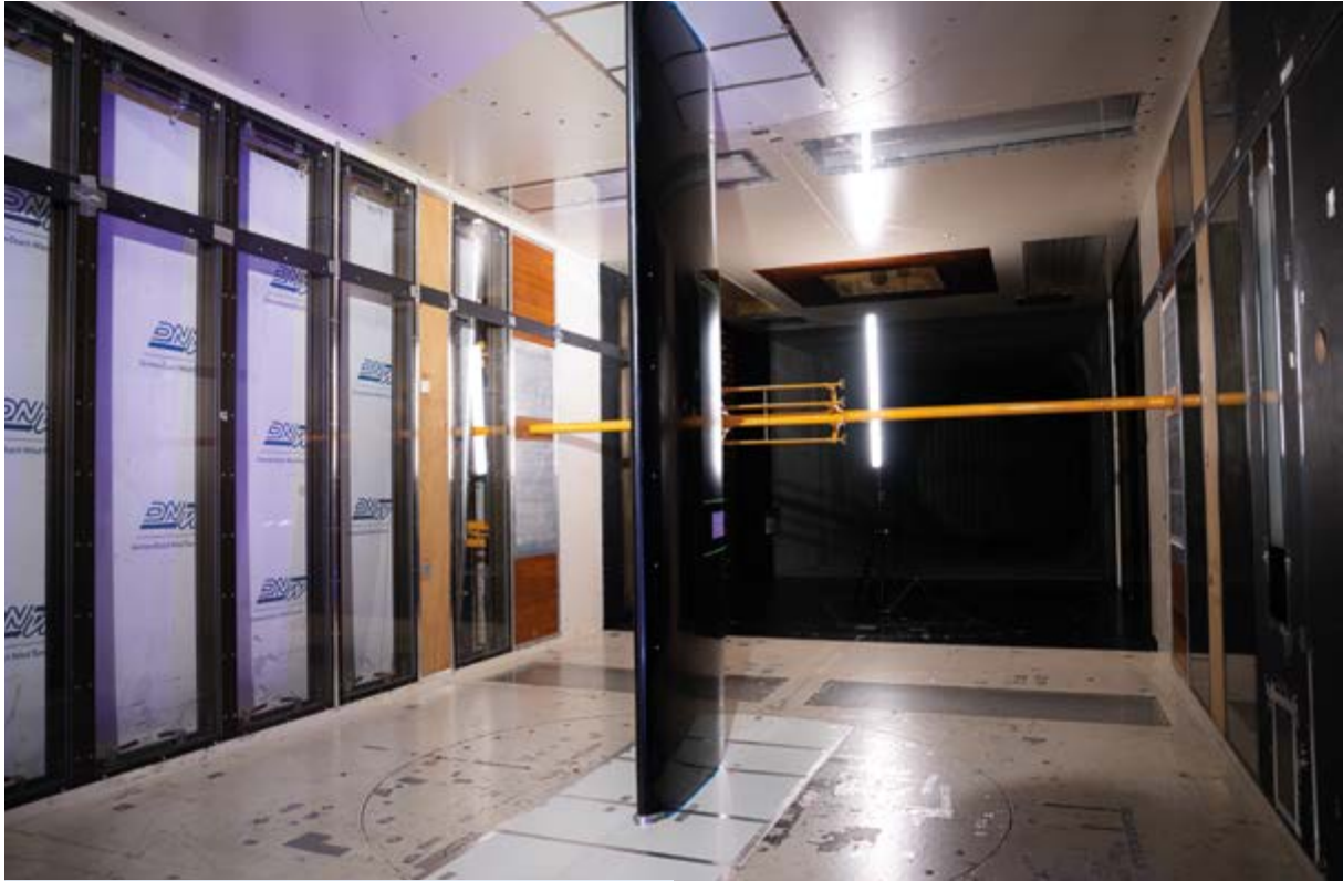
2D airfoil testing (Richting RVO TSH project)
