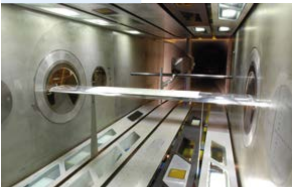
2D airfoil testing
