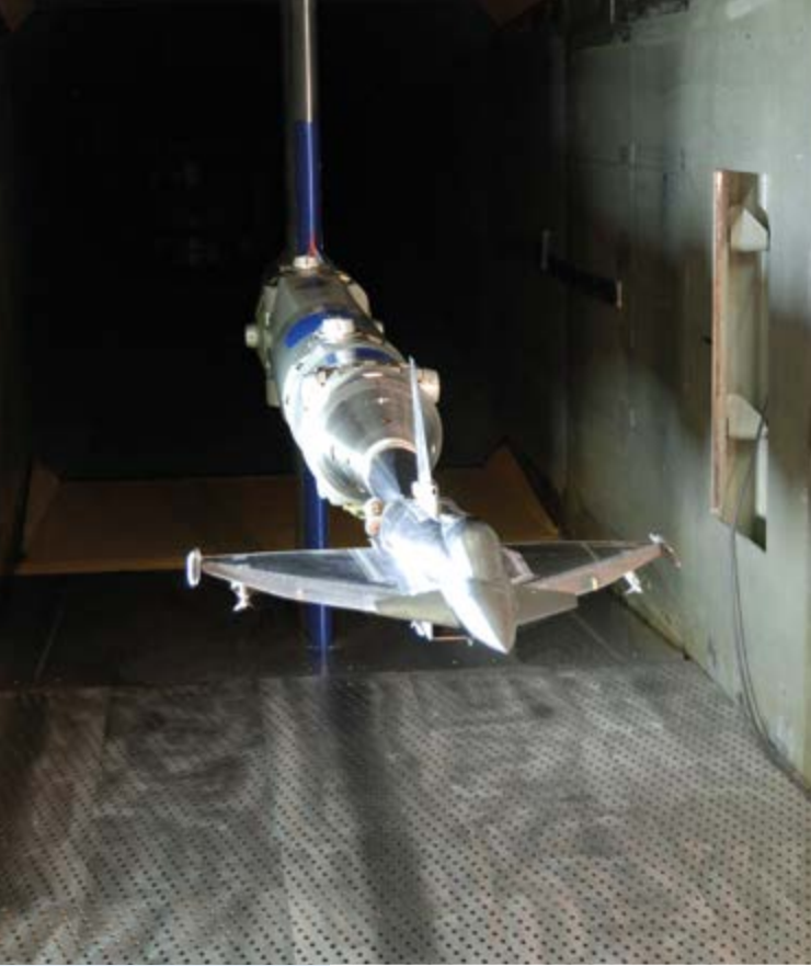
Fighter model testing (FA5 model ©Breitsamter@TUM-AER)
