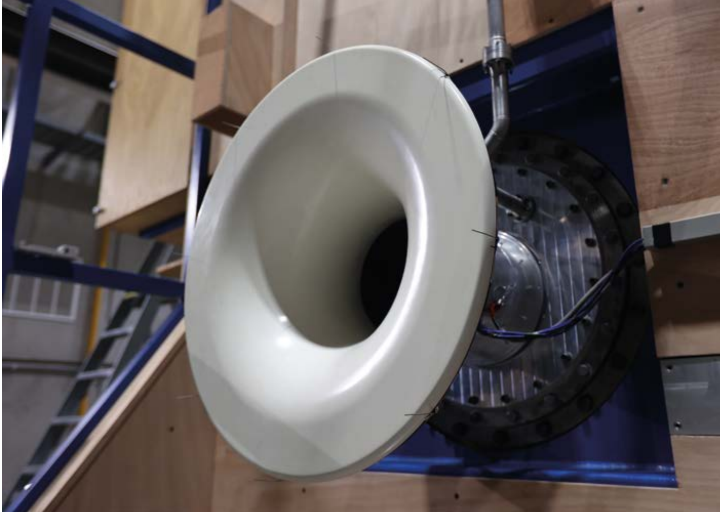
Bellmouth mass-flow calibration
