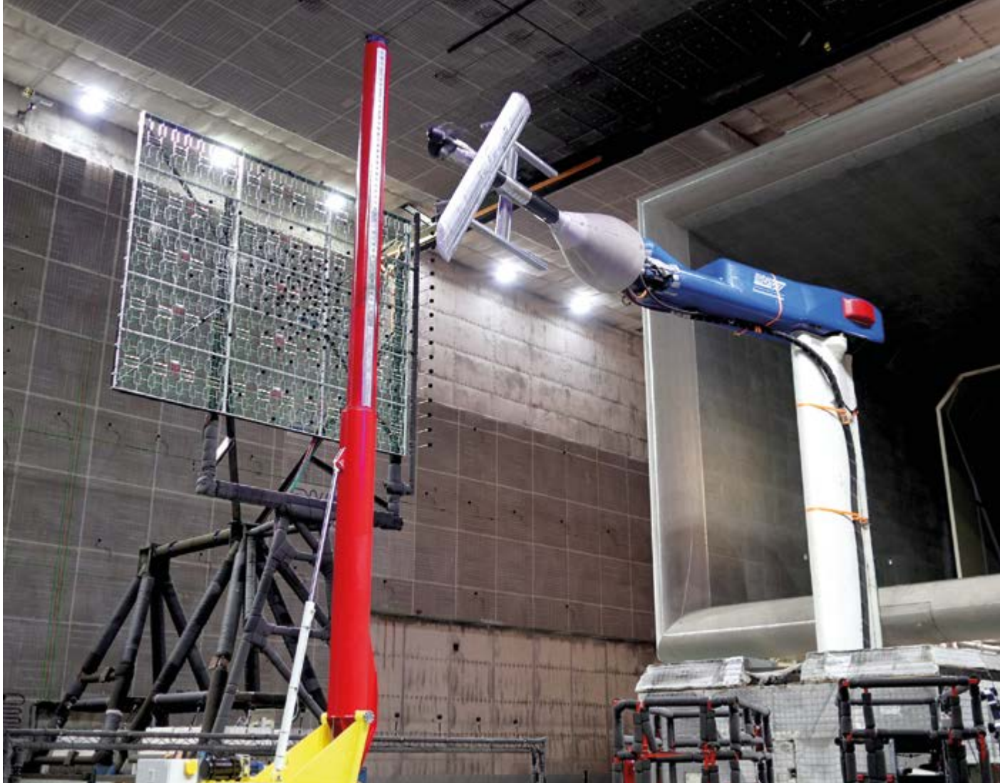
Open rotor performance and aero-acoustics
