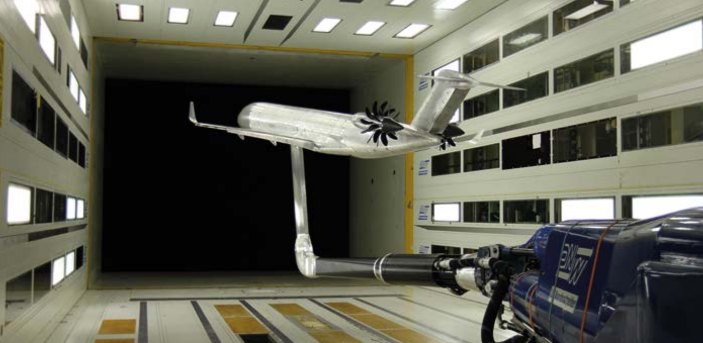
Propulsion integration test (L-CROR CTS Clean Sky project)
