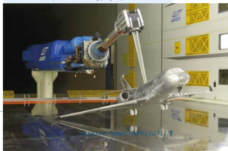
Business jet model in ground effect (PLAAT Clean Sky project)
