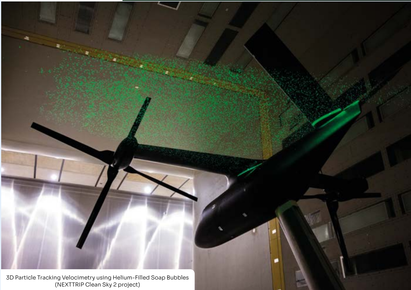
Particle Image Velocimetry (NIFTI Clean Sky 2 project)
