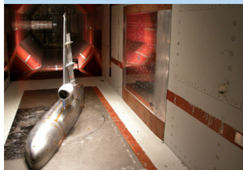
Figure 4 Acoustic measurements with a 9.24% scaled half-model of the Dornier-728.
