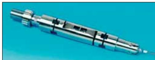
Figure 3: Free-to-roll DLR missile model mounted on a six-component piezo balance used in TWG
