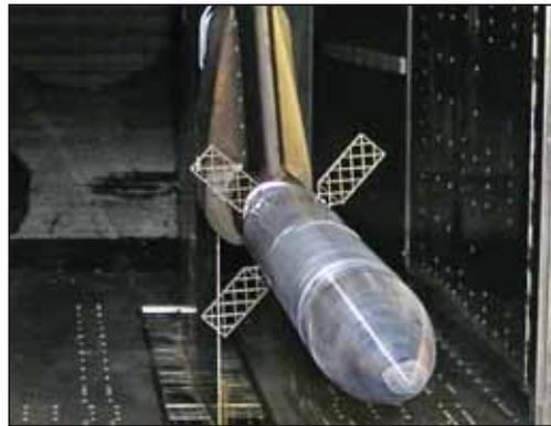
Figure 4: DLR missile model in the TWG
