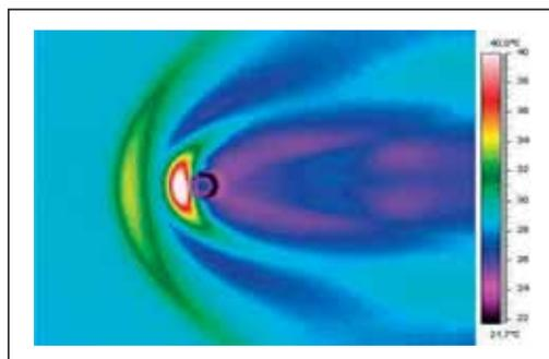
shows a top view of an infrared image of heat transfer on a model with a lateral jet at Mach 5 (flow coming from the left). The study aimed at analyzing the effects of various upstream devices on the flow characteristics.
