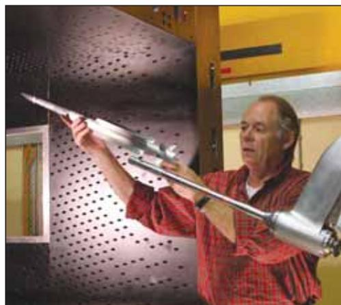
Figure 5: Mounting of an (air-to-air) missile model on a  $25^\circ$  cranked roll adapter in the TWG test section
