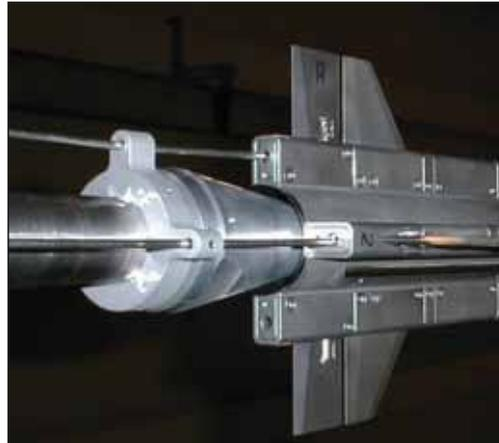
Figure 7: Throttling cone for adjustment of internal flow
