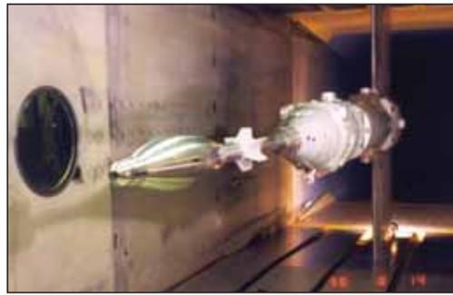
Figure 6: A model of an air-to-ground smart bomb in the HST
