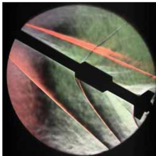
Figure 8: Schlieren picture of a missile in the TWG
