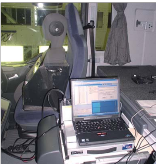
Figure 6: Dummy driver with ear microphones and data acquisition and processing equipment inside the truck cabin during LLF testing.
