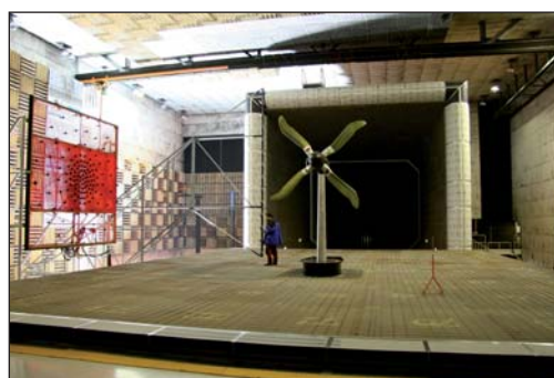
Figure 3: Downstream view of the LLF three-quarter open-jet test section with the tilt-rotor model in forward-flight mode, and acoustic instrumentation in place
