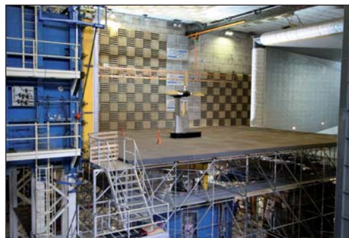
Figure 2: Side-view of the LLF three-quarter open-jet test section with the tilt-rotor model on the external balance in hover mode
