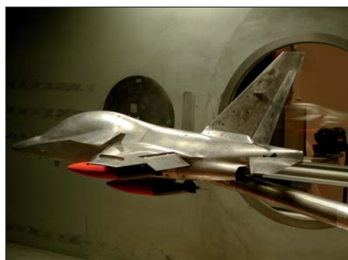
Figure 2: Three-quarter rear view of the M-346 model with external stores, mounted in the HST
