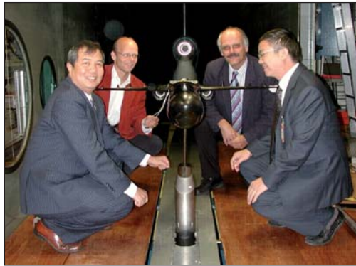
Figure 1: Guests from China inspect the small-scale ARJ21 model mounted inverted in the HST for ground interference assessments
