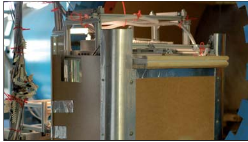
Figure 1: Generic convection cell for mixed convection studies in the open lock of the HDG
