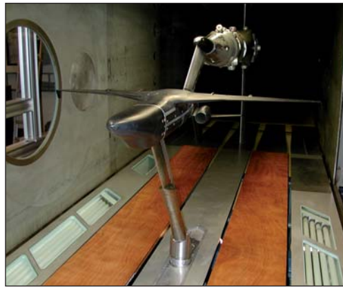
Figure 2: Test setup for support interference investigations with an IAI business jet model mounted upside down on a dorsal sting in the HST
