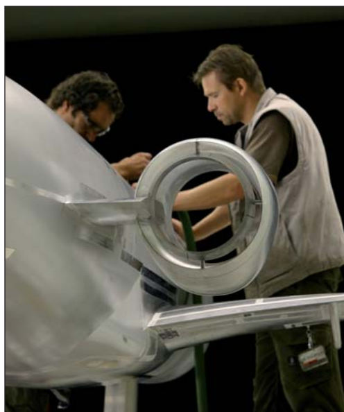
Figure 5: Through-flow nacelle fitted to the ARJ21 large-scale model
