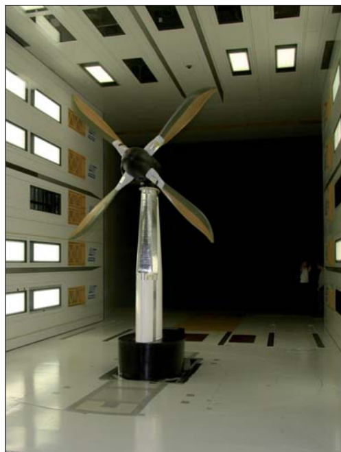
Figure 4: Tilt-rotor test setup for the ADYN whirl flutter tests in the LLF 6 m x 6 m closed test section
