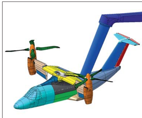
Figure 1: Schematic grid representation of the tilt-rotor model with dorsal sting support, for whirl-flutter analyses
