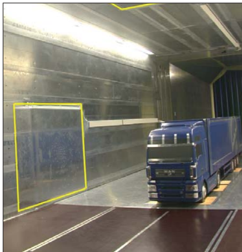
Figure 2: NWB test section with 1:4 scale TGX model truck and microphone wall arrays (outlined in yellow)
