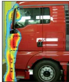
Figure 5: Projected source plot on the port side of a MAN truck-trailer combination in the 9.5 m x 9.5 m test section of the LLF
