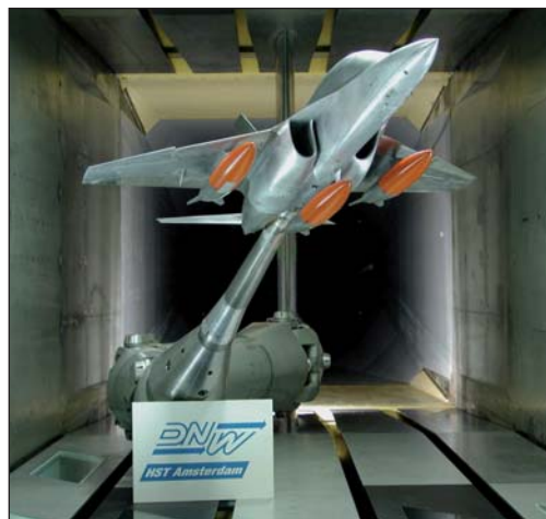
Figure 1: Test setup with the 1:10 scale M-346 model mounted on the articulated boom support in the HST
