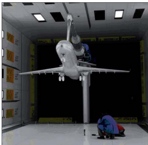
Figure 3: ARJ21 large-scale model mounted in the LLF above the ground plane with a dorsal sting setup
