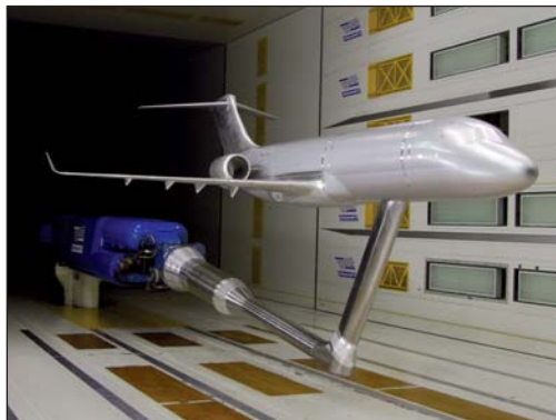
Figure 2: ARJ21 large-scale model mounted in the LLF with a ventral sting setup
