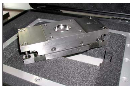
Figure 12: New Emmen box-type strain-gauge balance purchased for reduced-scale train tests in the HDG
