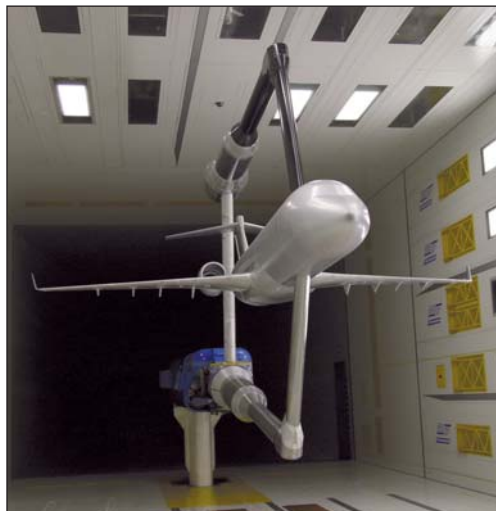
Figure 4: ARJ21 large-scale model in the LLF on a ventral sting and fitted with a dummy dorsal sting for support interference assessment
