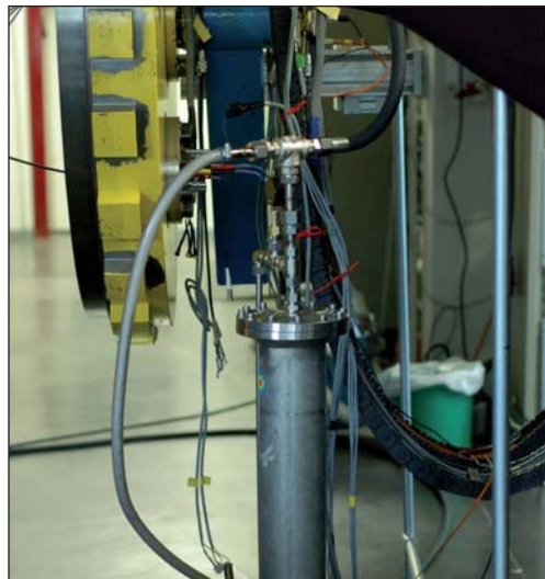
Figure 3: Fluidized-bed seeding generator
