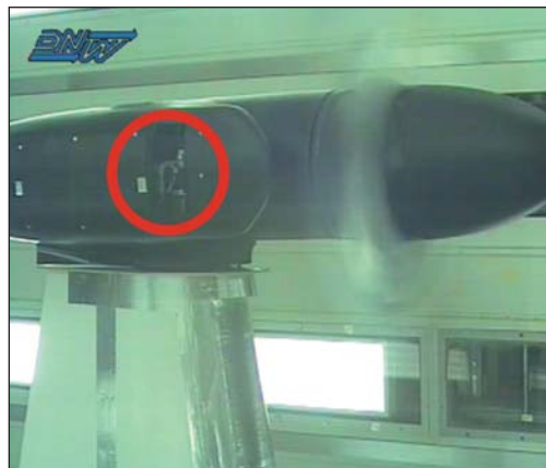
Figure 5: The tilt-rotor model's rotor-nacelle pictured during an ADYN whirl flutter test run with internal actuators (encircled) attached to the support structure
