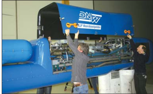
Figure 2: New LLF sting support fairing with the upper cover being removed
