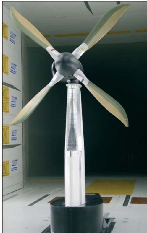
Figure 1: Tilt rotor model of the EU project ADYN in the 6 m x 6 m test section of the LLF
