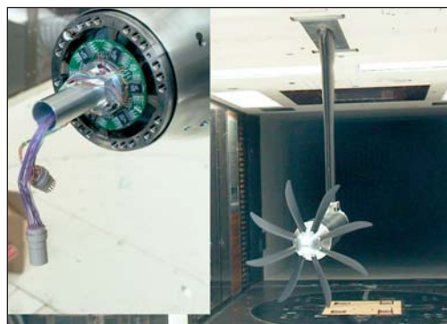
Figure 6: Set-up of the isolated propeller test in the LST; the insert shows a rotating shaft balances
