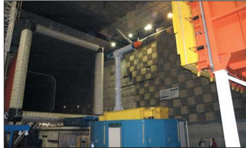
Figure 2: MEXICO PIV set-up. The wind tunnel flow is from right to left
