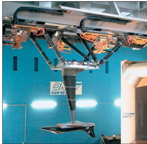
Figure 3: Aircraft model suspended from the MPM at the NWB
