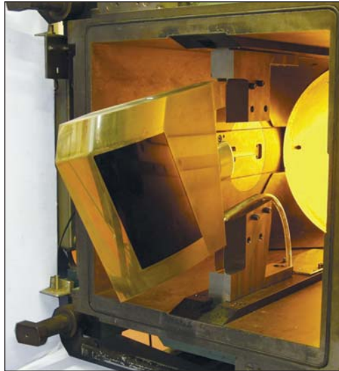
Figure 8: SUPERTRAC model in the test section of the RWG
