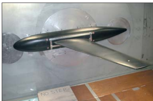
Figure 1: The UW-5006-NLF wing and fuselage installed in the HST
