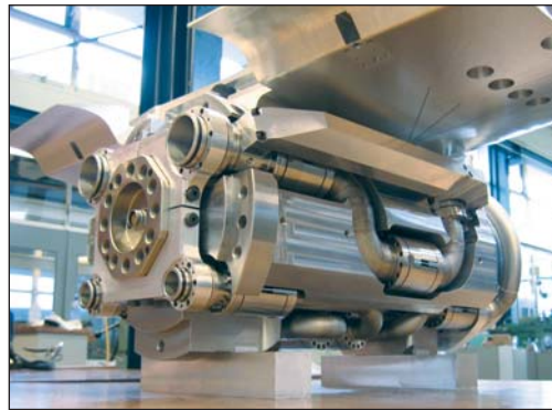
Figure 2: Airline bridges for the reduction of parasitic effects to the internal force and moment balance
