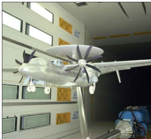
Figure 1: Model of the Advanced Hawkeye in the 8 m x 6 m test section of the LLF
