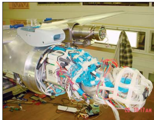
Figure 4: Impression of the complexity of instrumentation inside a wind tunnel model
